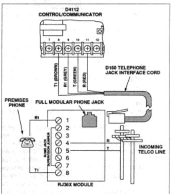
Figure 3: RJ38X WIRING
