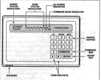
Figure 5: D420A COMMAND CENTER KEYPAD
