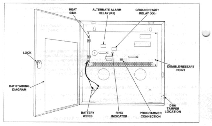
Figure 1: D4112 CONTROL/COMMUNICATOR ASSEMBLY
