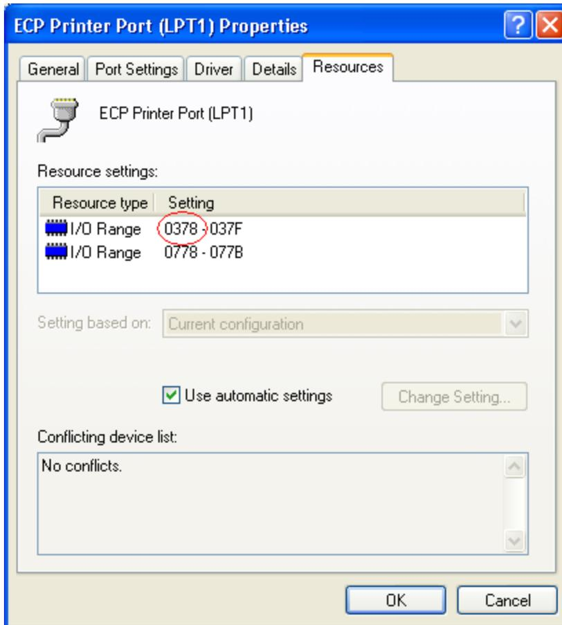
For many adapters the port address is shown under the resources of the Multi-IO adapter and not under LPT ports.
