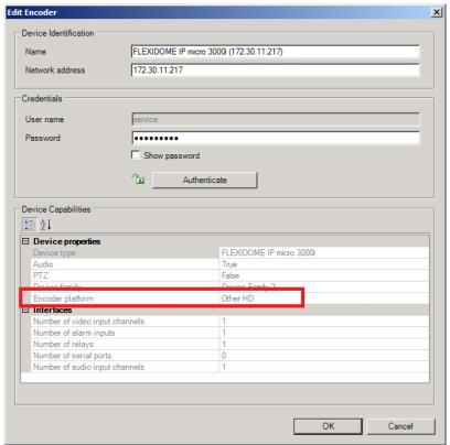
Go to the *Cameras and Recordings* page in the Configuration Client. The platform is detected as *Other HD*. Some codecs might not be recognized by the system.
