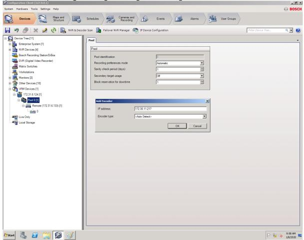
The camera can be manually added to the system. The encoder type should be on <*Auto Detect>*. After the camera has been added it might not be authenticated. Right click the camera to authenticate to the camera and enter the pre-configured username and password. Right click the camera and open the *Edit Encoder* dialogue to confirm the platform of the camera.
