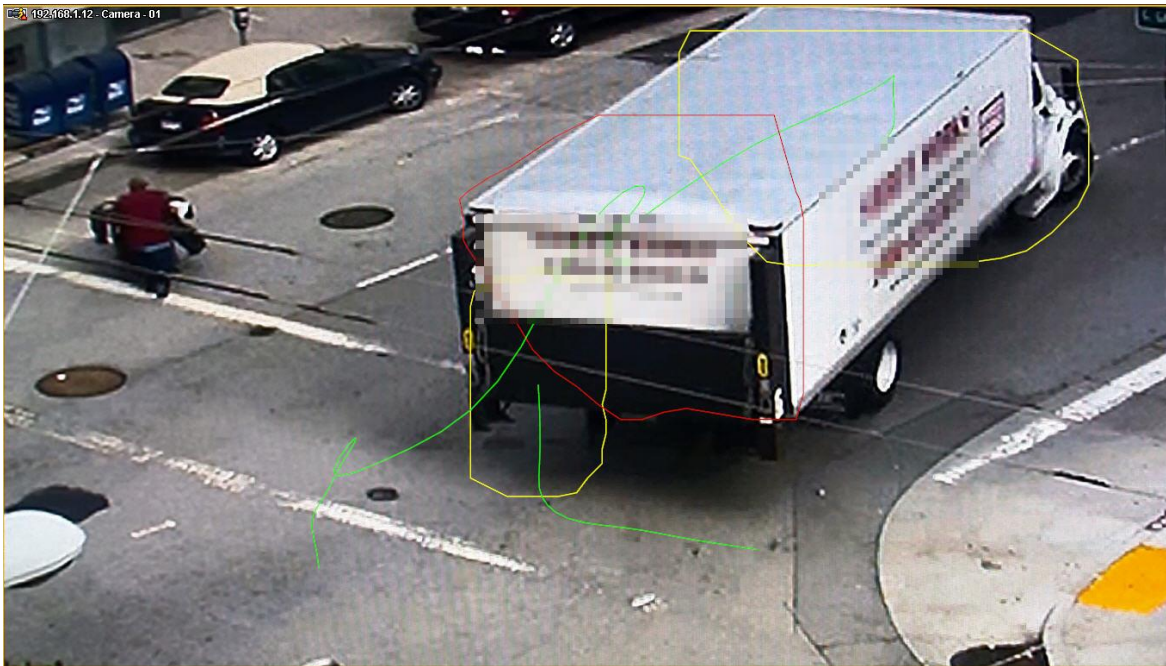
The truck is not correctly detected or classified because it is too large in the image
