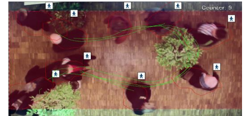
Counting people crossing a line (top) or currently inside a field (bottom). 3D people tracking mode allows to accurately separate close and slightly occluded people even in well-populated scenes
