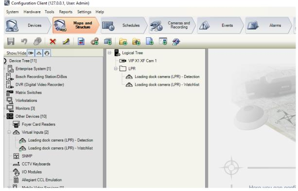
Trigger alarms (if necessary) for the related virtual inputs. The virtual input used for receiving all ANPR events will not be configured to raise an alarm. The virtual input which receives the watchlist events will be configured to raise an alarm.
