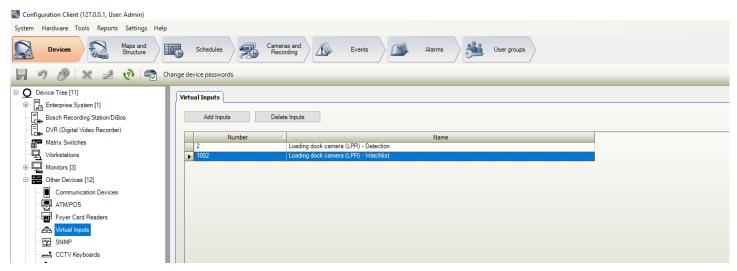
Add the virtual inputs to the logical tree. It is recommended to add, per ANPR camera, one virtual input which receives all ANPR events and one virtual input which only receives and event when a watchlist is triggered.
